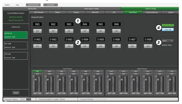
The Auto mixer automatically reduces the level of a microphone when it is not being used. Consequently it lowers the rumble, reverberation and other extraneous noise that occur when several microphones operate simultaneously.
