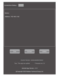
5). Select the IP address applied on the unit which needs updating, Click "connect" box, The green will light for "connection-status" indicator.
