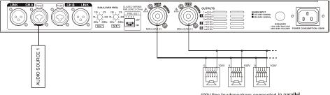
100V line loudspeakers connected in parallel
