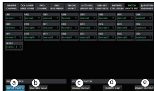
a). Input Patch: Different input signal source can be selected for each channel, the Analog 1~24 or Digital 1~32 can be selected as input channel.
