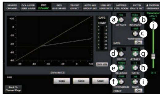
a). Touch it to set the time for the gate to change from closed to open and It can be set from 0.5 to 200 ms. Although faster attack is very important for percussion instrument. It maybe take much more time to attack the slower rising signal like voice and bass guitar so that the click noise can be heard easily from each noise gate based on the fast attack time. So proppriate ATTACK settings is an effective way to avoid click noise.
