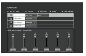
a) Input Source: Click the drop-down arrow to select input source from None, Input1-6, D-Input 1-8.
