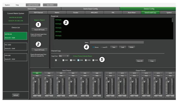
This menu is used to manage the backup parameters. These data can be stored directly in the internal memory of host as a preset. Its memory contains a total of 24 presets.
