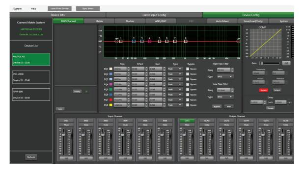
Note: Except "Expander/Gate" part, the same menu as DSP input channel's applied. The EQ parameters here is equipped with 8 bands, Details as introduction of DSP input channel.
