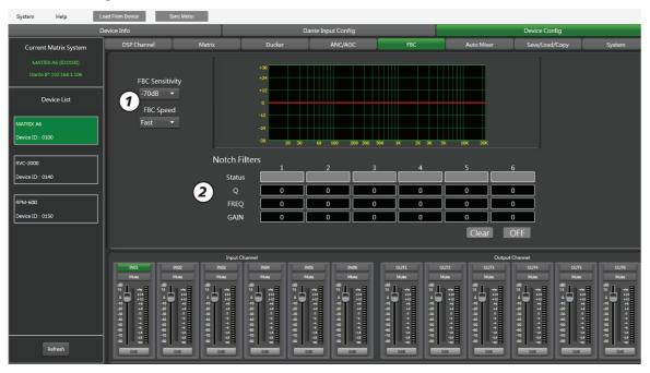
**FBC(Feedback Canceller)** is a function which eliminates feedback automatically. Feedback occurs unexpectedly in a system where there are microphones and speakers nearby one of the other.
