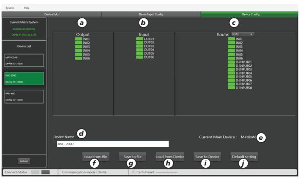
a). Output: Total 6 output channels from CH1 to CH6. Green box means available channel, And grey box mean disable channel.
