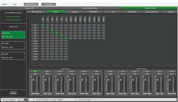
This part of the software is used to route inputs through a graphical representation as a matrix. By clicking on the gray boxes several inputs can be assigned to several outputs. If the connection is active the box turns green, otherwise it remains gray. The matrix can route 14 input signals to 14 separate outputs. One talks about a  $14 \times 14$  matrix.
