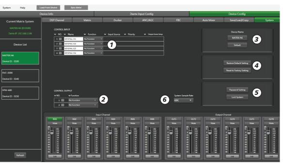
1). CONTROL INPUT: There are total 4 external trigger ports from controlinput1 to controlinput 4. Once trigger command received sucessfully, The corresponding box of NO.1~NO.4 will light, It means the preset functions take effects on the corresponding trigger port.
