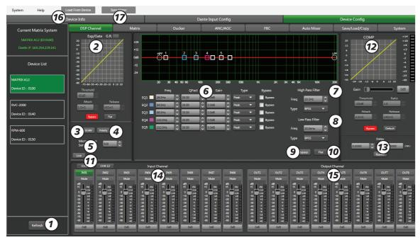
Double click "MATRIX A12" in device list to enter the DSP input-channel configuration interface of PC software.
