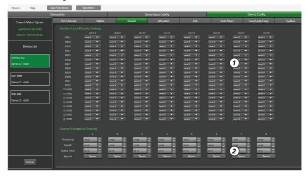
The principle of the Ducker is to attenuate one or several channels when priority signals are activated. The main applications are automatic speech for conference or priority messages. E.g.Use the host microphone signal to control the background music volume. The host automatically reduces the background music volume when speaking. After the speech, the volume is automatically restored.
