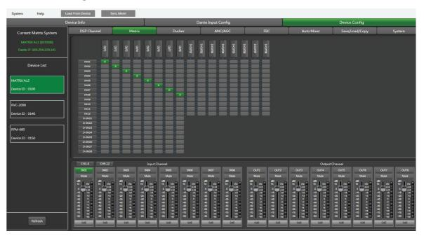
This part of the software is used to route inputs through a graphical representation as a matrix. By clicking on the gray boxes several inputs can be assigned to several outputs. If the connection is active the box turns green, otherwise it remains gray. And the volume is adjustable. The matrix can route 20 input signals to 16 separate outputs. One talks about a 20 x 16 matrix.
