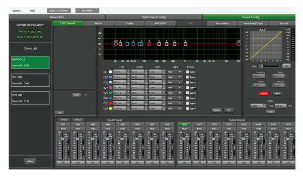
**Note:** Except "Expander/Gate" part, the same menu as DSP input channel's applied. The EQ parameters here is equipped with 8 bands, Details as introduction of DSP input channel.
