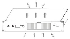
Air flow in D series Digital Amplifier: Cool air is drawn into the left of the amplifier by the cooling fan. Warm air exits the right of the amplifier.
